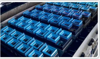
Are you still manually wiping your print head? This automated print head cleaning and capping technology is a consistently controlled process which reduces manual operator intervention and reduces waste.
