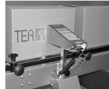
The C-Series printers are capable of printing up to four lines of text at once (depending on the model used), each line containing up to 40 characters. Text heights range from 10mm to 68mm. Each line (or lines) of text printed at once is known as a “message”. 50 separate messages can be stored in the printer’s memory. Once input, these messages can be recalled for printing at the touch of a button and are entirely unaffected by power loss.
