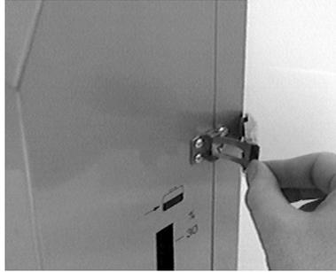
To close the ink compartment door, reverse this procedure. Hook the catch around the fastening on the rear of the base unit and press it in place. Take care not to trap the ink and air lines when closing the door.
