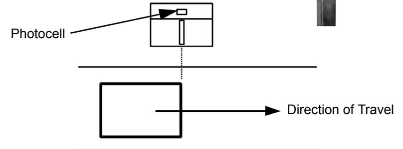
The system then allows a short time delay to enable the item to be carried on past the print head. This delay depends on the speed of the conveyor and the length and position of the message and is set by the operator for each message.
