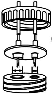
*Note: Ensure that the large and small probes go into the correct holes.*
