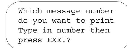
Type in the number of the message to print then press the ENTER key. The next time the photocell is triggered the selected message will be printed.
