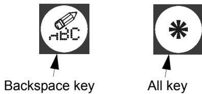
The ALL key is used in many functions to select all the messages in the printer's memory.
