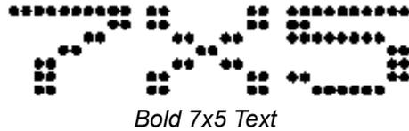
To print in bold, enclose the relevant part of the message in the curly brackets which can be accessed by holding down
