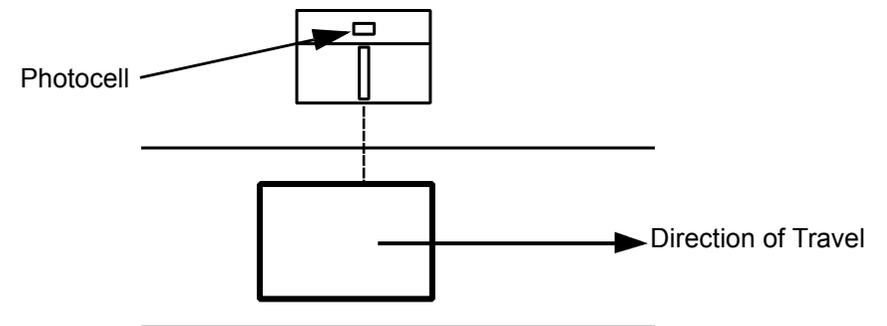
When the item is at the correct position in respect to the print head, the desired text is printed by repeated triggering of the solenoid valves.
