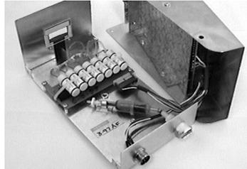
*Lift off the top of the chassis*
