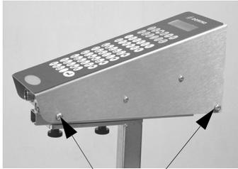
*Unscrew and remove the print head screws*
