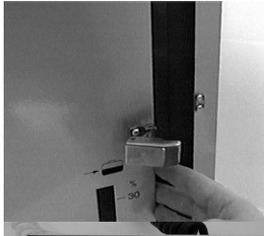
This photo shows the interior of the three litre base's door. The captive ink bottle cap can be clearly seen hanging from its connecting air and ink tubes. All the base unit's electronics are located behind the panel in the door.
