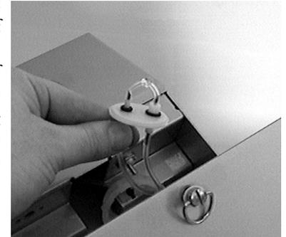
**WARNING:** If replacing an empty ink bottle, remember to switch the power off and press the pressure release valve before unscrewing the old bottle.
