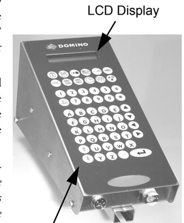
The keypad is in three sections. Pressing any of the special icon keys at the top accesses the appropriate function as detailed in the Programming and Printing
