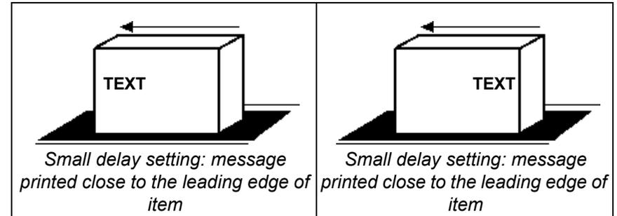
Delay is normally set for each individual message since different messages will be of different lengths. Long messages may need shorter delay times than brief messages. The delay value used will also depend on the speed of the conveyor - faster conveyors may need lower delay times.
