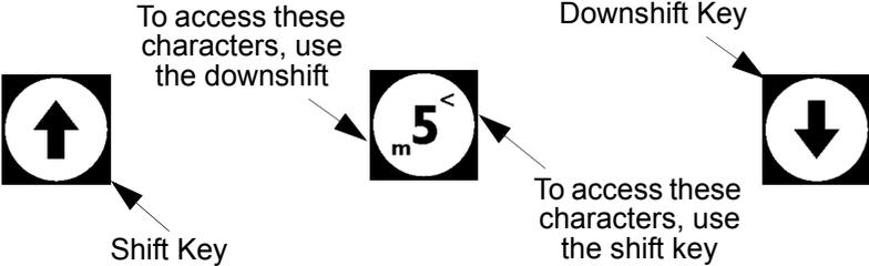
The DOWN SHIFT key is used in combination with the number keys 1 to 6 to enter the lower case characters displayed in red in the bottom left hand corner of the key.
